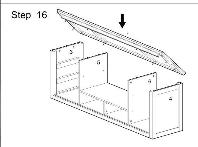
Attach the top panel (1) to the assembly from the previous step using cam bolts and dowels as guides.
